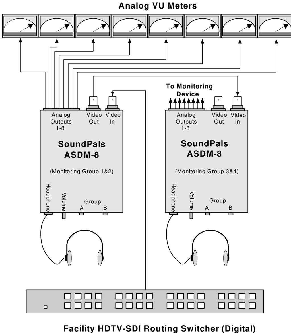
In this application, the facility's SDI / HDTV-SDI routing switcher is fed to the first ASDM-8 SoundPal, which is selected to monitor Group 1 & 2 and drive the eight Analog Meters. The video signal is then fed from the active video output connector to the second ASDM-8 SoundPal which is selected to monitor Group 3 & 4. The eight analog audio signals are then fed to a monitoring
